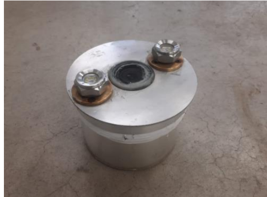
Figure 1 The first iterative attachment fabrication with light, camera and tempered glass attached
